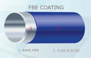
FBE Coating has been used as a standard in industries for protection against corrosion. FBE coatings have good handling characteristics; they are flexible and resistant to soil pressure. These are used in pipeline projects that have normal requirements and do not have harsh conditions.
